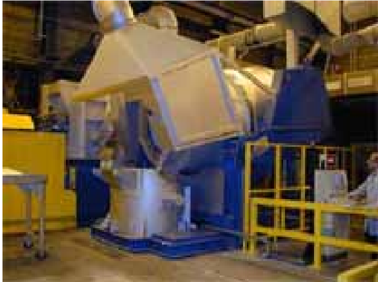
Dross Engineering Dross 200 tap-out
